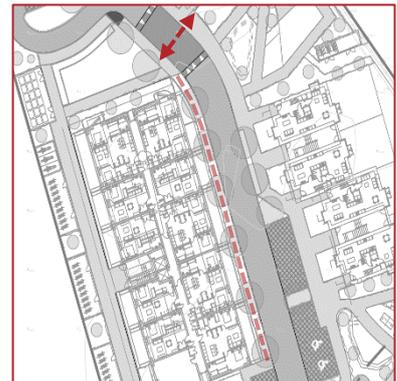
This could lead to visually, and mobility, impaired pedestrians being unable to safely and independently navigate the road layout and being stranded within the footpath at this location. Pedestrians may continue within the verge where there is an increased risk of trips and falls or cross the carriageway to the opposing footpath where there is an increased risk of being struck by a vehicle should drivers be less attentive to pedestrians crossing away from formal crossing points.
